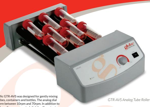
The Globe Scientific GTR-AVS was designed for gently mixing a wide range of tubes, containers and bottles. The analog dial can be set anywhere between 10rpm and 70rpm. In addition to a rolling motion, the rollers are mounted slightly off-center to rise and fall in a "see-saw" fashion. These two motions ensure your samples are thoroughly mixed for optimal homogeneity. The six rollers can accommodate up to 8.8lbs or ten 15ml / 50ml centrifuge tubes.
