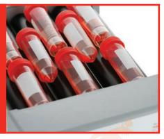
The six roller configuration can accommodate up to ten 15mL or ten 50mL tubes and is compatible with a variety of other tube sizes
